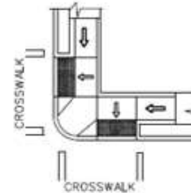
EXAMPLE PLACEMENT AT INTERSECTION WITH BUFFER STRIP
